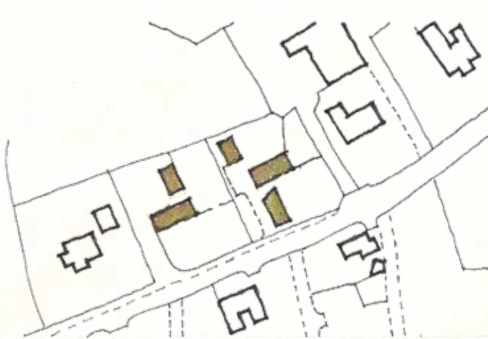
PLAN SHOWING WELL SITED AND SCALED 2 HOUSE INFILL. NOTE HOW THESE REFLECT TRADITIONAL SITING PATTERNS
