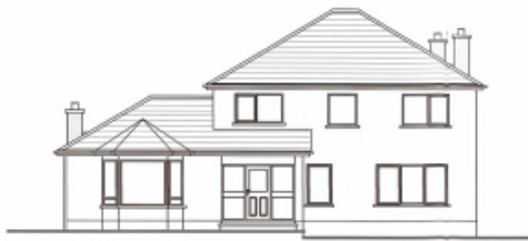
EXISTING REAR ELEVATION
