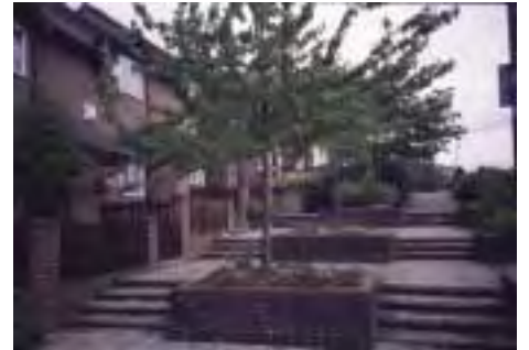
Footpaths serving dwellings should be accessible to people with disabilities. The use of steps should therefore be avoided.
