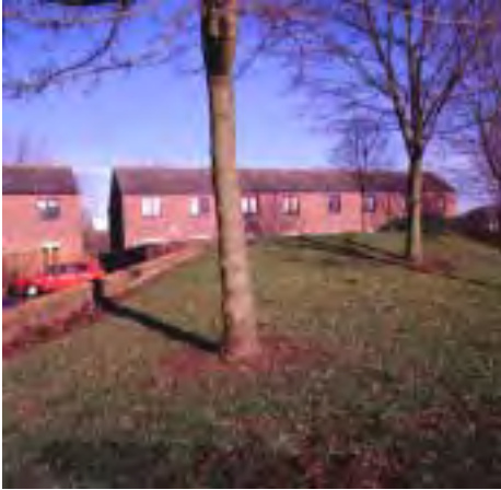
Mounding and planting can help alleviate the adverse effects of exposure and ameliorate noise nuisance.
